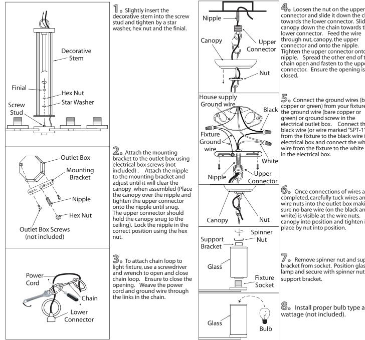
connector and slide it down the chain towards the lower connector. Slide the canopy down the chain towards the lower connector. Feed the wire through nut, canopy, the upper connector and onto the nipple. Tighten the upper connector onto the nipple. Spread the other end of the chain open and fasten to the upper connector. Ensure the opening is
